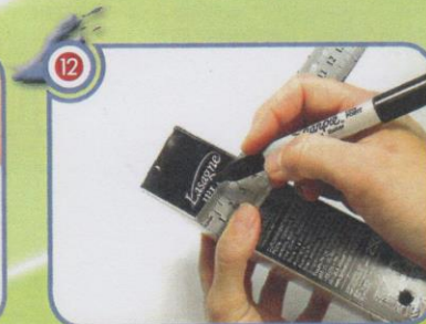
Measure four spots onto the bottom corners of each side of the box. Make sure the spots are in the same place on each side. Alternatively, make a template (see next step).
